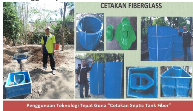
Figure 7. Use of Appropriate Technology "Fiber Septic Tank Mold"
